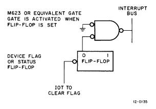
Figure 5-11. Program Interrupt Request Signal Origin
