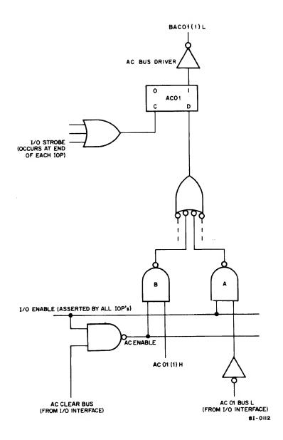
Figure 5-8. Accumulator Input or Output
