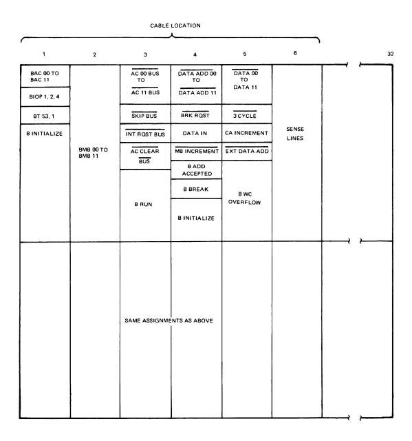
Figure 5-30. I/O Cable Connections
