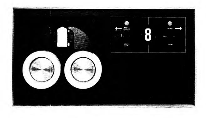
Figure 2-5. TU55 Tape Transport Control Panel
