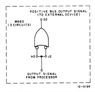
Figure 5-26. M660 Terminated Bus Driver Output Circuit
