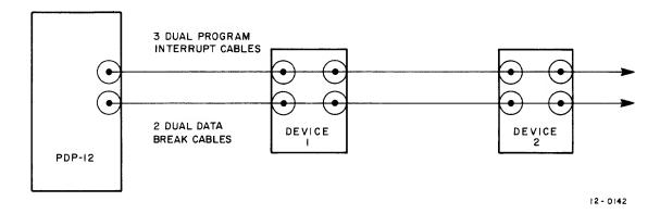
Figure 5-29.\ I/O Bus Configuration
