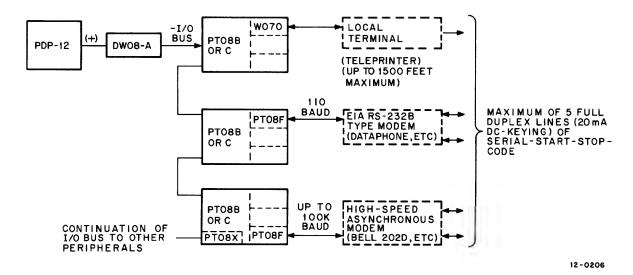
Figure 6-3. PT08 Equipment Configurations
