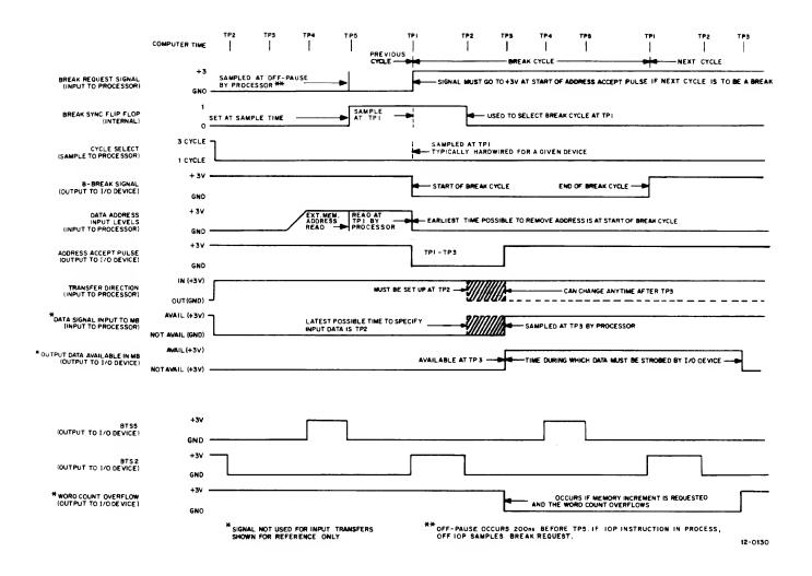
Figure 5-17. Single Cycle Data Break Input Transfer Timing Diagram
