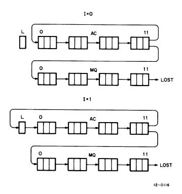
Figure 3-7. Rotate Right
