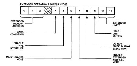
Figure 3-19. Extended Operations Buffer Bit Assignments
