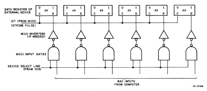
Figure 5-10. Loading a Six-Bit Word into an External Device from the Accumulator
