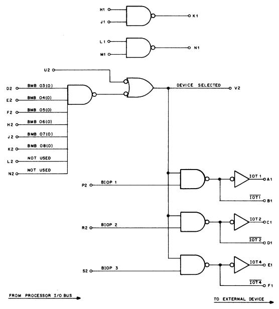
Figure 5-27. M103 Device Selector Logic Circuit
