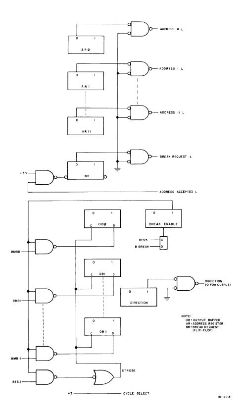
Figure 5-20. Device Interface Logic for Single-Cycle Data Break Output Transfer
