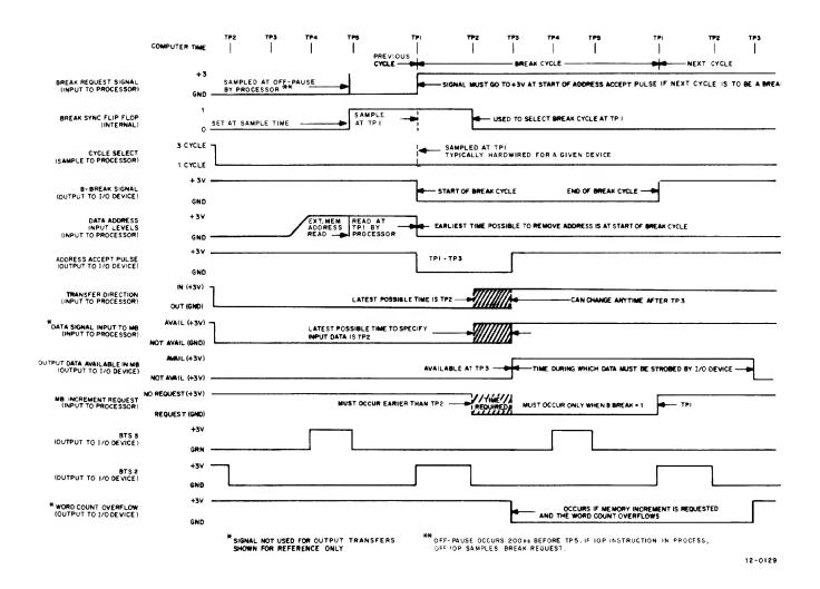
Figure 5-19. Single-Cycle Data Break Output Transfer Timing Diagram
