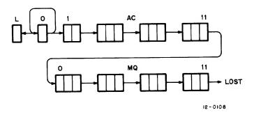
Figure 4-8. Shift Path for ASR
