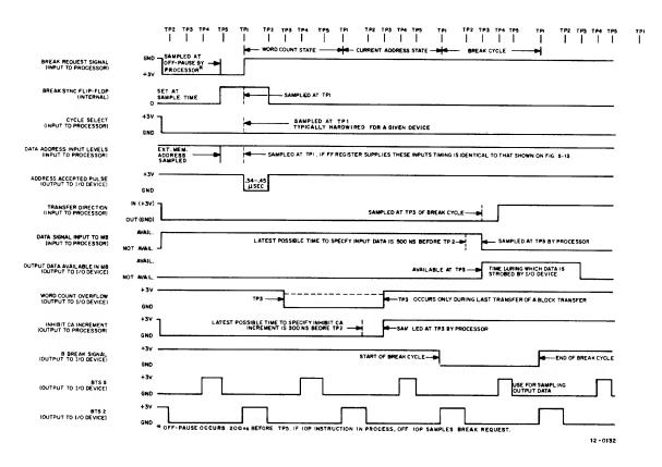
Figure 5-22. Three-Cycle Data Break Timing Diagram
