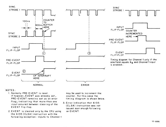
Figure 6-8. KW12-A Timing Diagram
