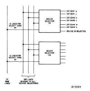
Figure 5-5. Generation of IOT Command Pulses by Device Selectors
