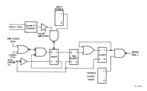
Figure 6-7. Simplified Input Synchronizer Logic Diagram
