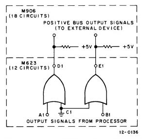
Figure 5-25. Typical M623/M906 Positive Output Circuit
