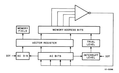
Figure 5-14. Vector Flow Diagram
