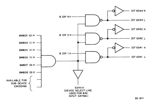
Figure 5-6. Typical Device Selector (Device 34)
