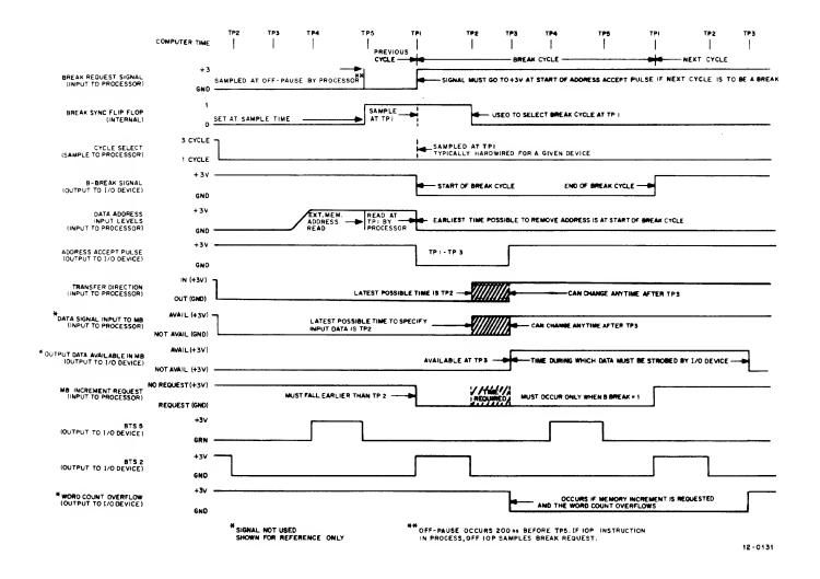
Figure 5-21. Memory Increment Data Break Timing Diagram
