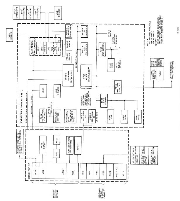
Figure 1-1. PDP-12 Functional Block Diagram
