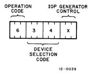
Figure 5-2. IOT Instruction Decoding
