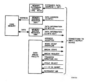
Figure 5-16. Data Break Transfer Interface Block Diagram
