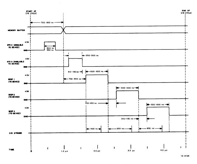
Figure 5-4. Programmed Data Transfer Timing
