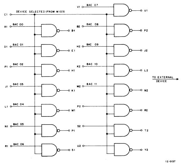
Figure 5-28. M101 Bus Data Interface Logic Circuit
