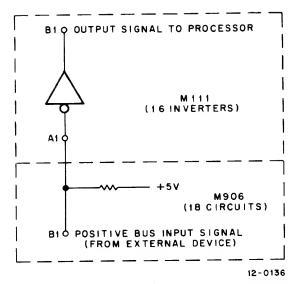
Figure 5-23. Typical M111/M906 Positive Input Circuit
