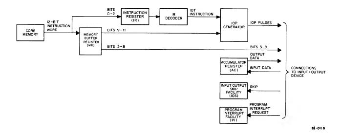
Figure 5-3. Programmed Data Transfer Interface Block Diagram
