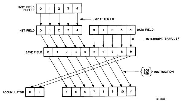
Figure 3-10. Data Path: IB, IF, DF, and AC
