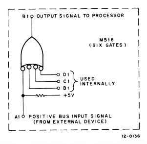
Figure 5-24. Typical M516 Positive Bus Receiver Input Circuit
