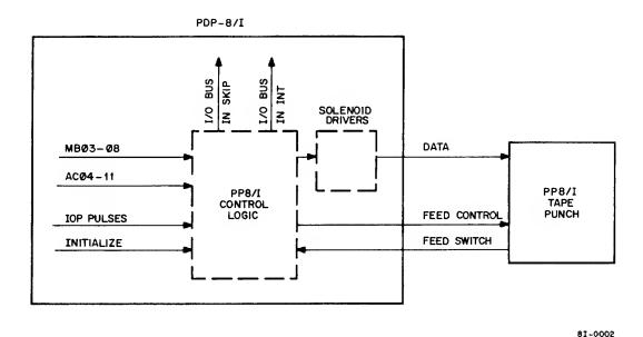
Figure 2 Block Diagram PP8/I Paper-Tape Punch
