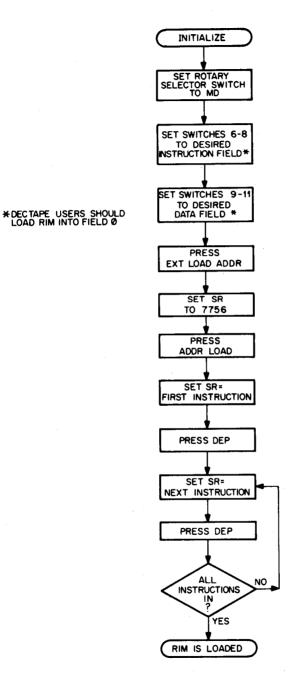
Figure A-1. Loading the RIM Loader
