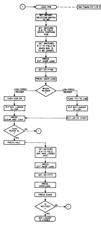
Figure A-3 Loading the BIN Loader
